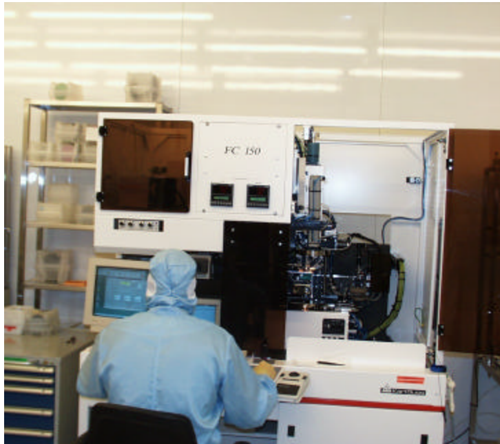
Suss MicroTec FC150 Flip Chip Bonder with both Universal and Solder Reflow Bonding Arms.
