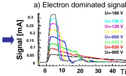
Electrons drift from a high to a low electric field
