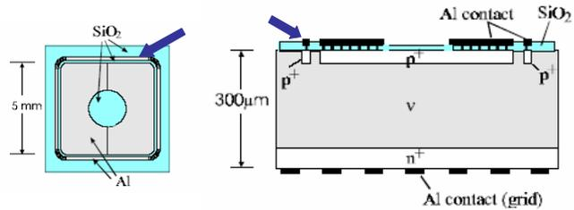
• 660 nm Red laser illuminates the front of the detector, penetration depth ~few μm
