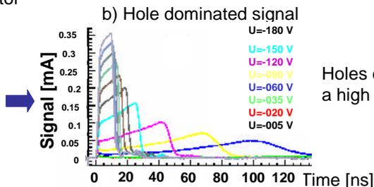
Holes drift from a low to a high electric field
