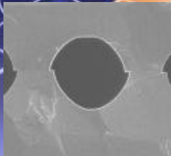
bonded wafer pair problem: misalignment
