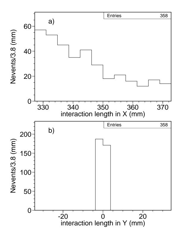
Figure 3: Position in X (up) and Y (down) where the photoelectric effect takes place for events with no other interaction.
