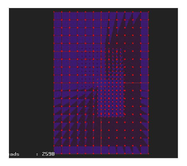
Figure 2: XY view of one PET module without the readout system. In the figure it is only shown the  $12 \times 18$  matrix of scintillator cystals.
