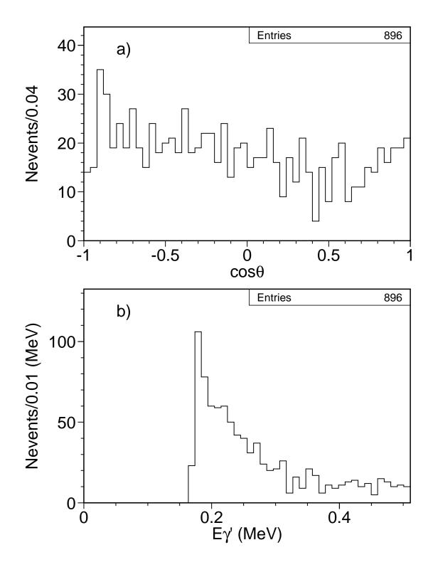
Figure 7: a)  $\cos \theta$  distribution after the Compton interaction for events in which there is a Compton and then a photoabsoption. b) Energy of the scattered photon after the Compton for the same envents.
