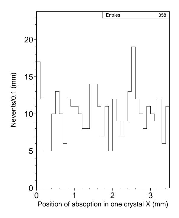
Figure 5: Position in X (up) and Y (down) where the photoelectric effect takes place in the crystal.
