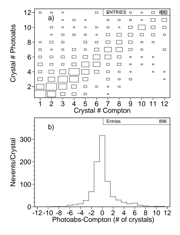
Figure 8: a) Number of crystal where the photoabsorption takes place versus the number of crystal where the Compton occurs in X for 1c+1pe events. b) Difference in number of crystals between the position of the photoabsoption and the Compton in X.
