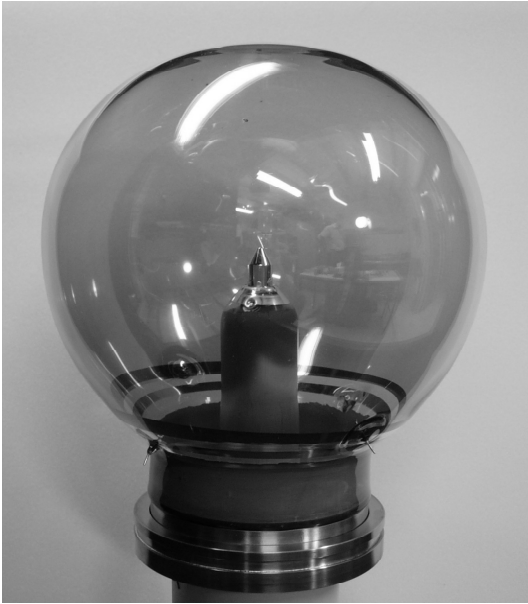
Fig. 1. Photo of the X-HPD with conical LYSO crystal anode.
