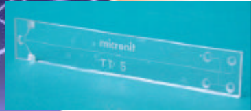
glass chip for capillary electrophoresis with end-column integrated conductivity detection
