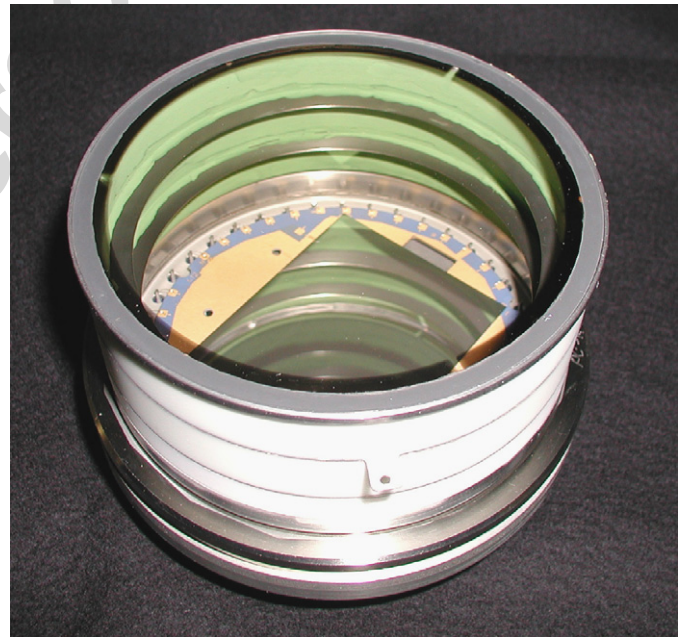
Fig. 3. Photograph of the sealed PET-HPD prototype tube. The Al-coated Si sensor is clearly visible.
