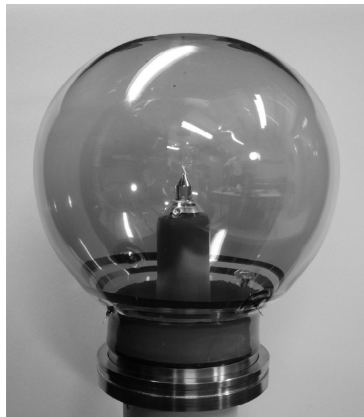
Fig. 2. Photo of the X-HPD with conical LYSO crystal anode.
