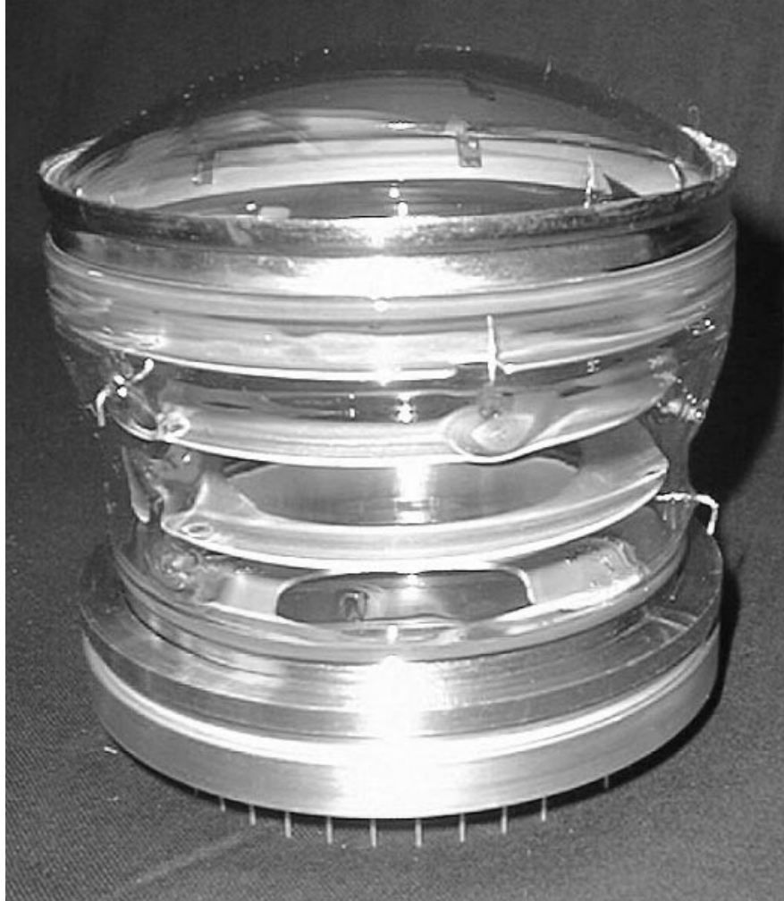
Fig. 2. Photograph of a sealed Pad HPD with bialkali photocathode and integrated readout electronics.
