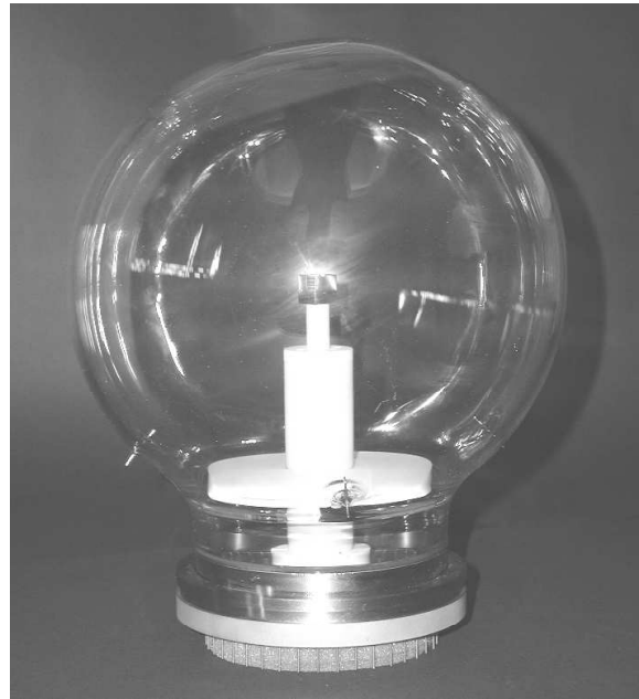
Figure 2. Photograph of the 'dry' assembly of the half scale prototype HPD.
