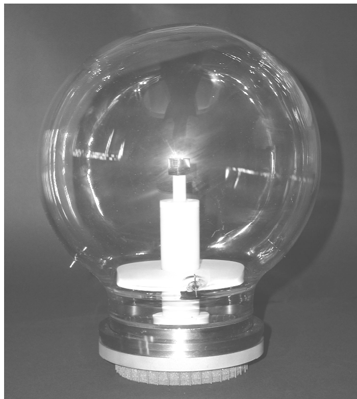
Figure 14: Schematic view of the optical module (top), photograph of a half-size prototype of the HPD (bottom).
