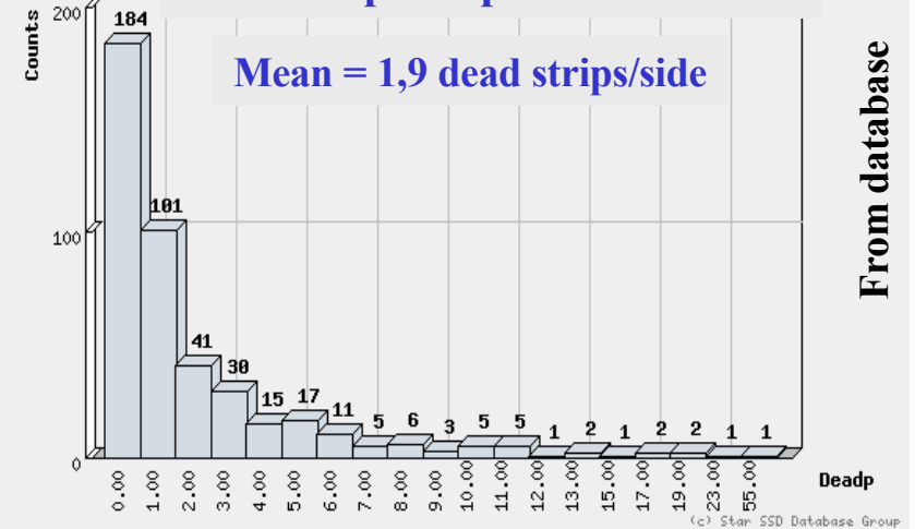
Dead strips on n-side /detector
