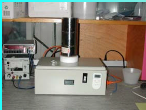
3 Furnaces for Si treatment
